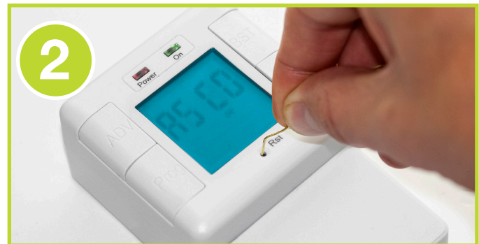
2 Reset the timer before programming for the first time by pressing the RST button underneath the display using a pointed object after charging.
