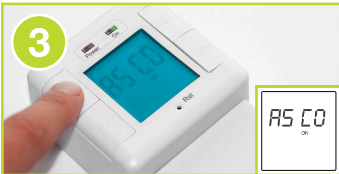
3 Use the ADV button to change between on and off for automatic summer time adjustment (Automatic Summer Change Over).
