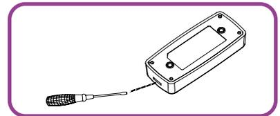
3. Offer the push button backing up to the wall and drill holes. If fitting to masonry, use a 6mm drill bit, as per the depressions and securing by using the supplied rawl plugs and screws. If fitting directly to the woodwork, use a 2mm drill bit and screw directly into frame or use the provided sticky pad.
