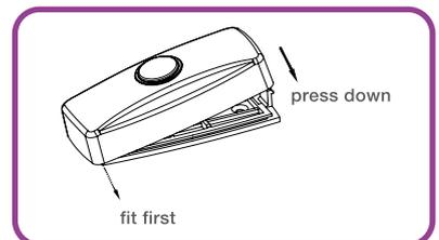
6. Identify a suitable position for the door chime within the recommended range and plug in. The socket is easily accessible. The door chime and push button is only suitable for mounting at heights <2m.
